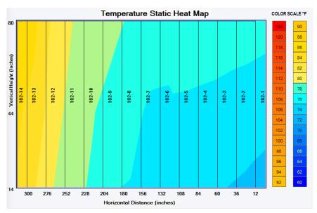
This Static Temperature Map shows the temperature distribution of Aisle 102, which contains 14 racks. This map shows hot spots at Rack 102-14, Rack 102-13 and Rack 102-12, where temperatures exceed 80.6°F
